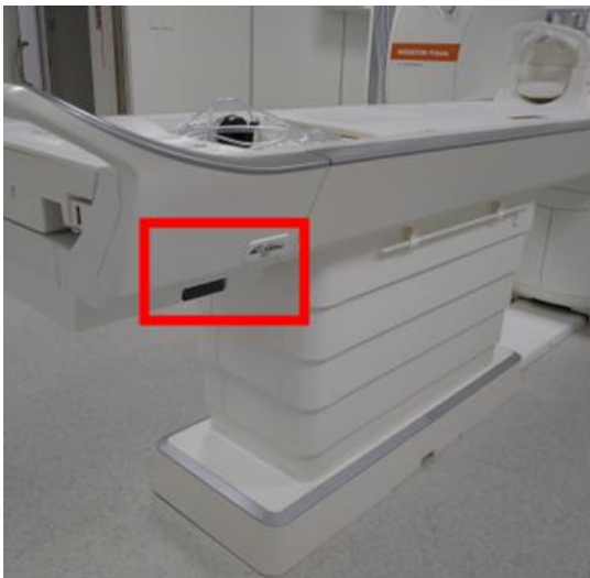
Figure 7. Location of emergency release handle
